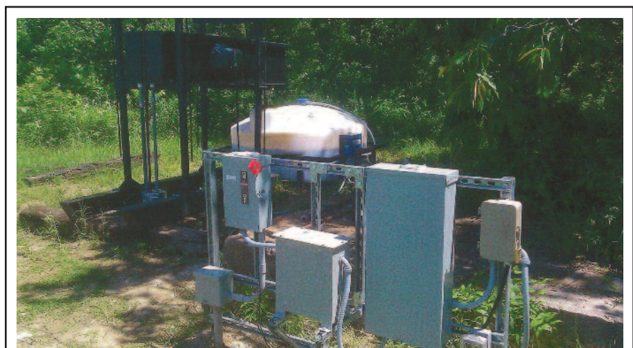
This system from Tokata Oil Recovery Oil Inc. uses oil-attracting, water-repelling materials to produce oil from marginal wells. Tokata says the system requires 5 percent as much electricity as a conventional pumpjack and can eliminate the need for separation equipment.
